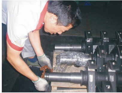
Picture 3-3: Installation of Bearing and Blade Rest
