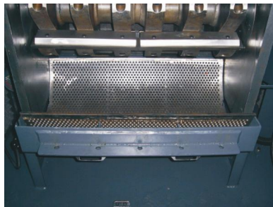
Picture 4-3: Close the screen bracket; the regrind storage bin and the feeding hopper
